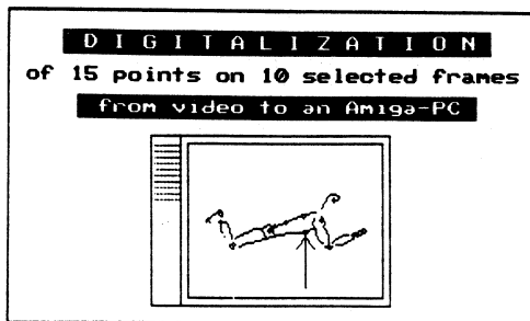
Fig. 13 : Presently, for a fast and inexpensive movement analysis and advice, video images can be overlaid onto a PC-screen (Amiga) to be digitized using a mouse.
